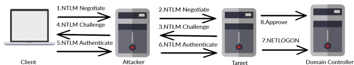
Figure 3: Relay attacks abuse credentials by intercepting and relaying valid challenges and responses in Windows NT LAN Manager (NTLM), Server Message Block (SMB) and other protocols.
